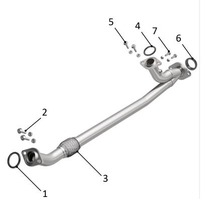
(Carefully read all instructions before installation) Disconnect the vehicle's battery before removal of the OEM exhaust system. This will prevent electrical accidents and will reset the computer if it applies to the vehicle. Remove existing front pipe from the vehicle. Only remove parts that will be replaced. Clean existing flange with a wire brush to ensure proper sealing.
